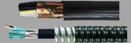
CIC / ACIC Single or multiple individually shielded pairs or triads, overall cable shield with PVC jacket. Optional armour and outer jacket.
