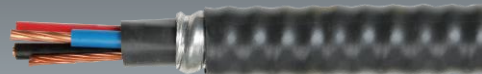
TECK90 Armoured and jacketed (inner/outer) cable with multiple XLPE-insulated Cu conductors + bare Cu ground
