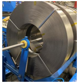
1. Aluminum strip is inserted into the machine in large rolls
