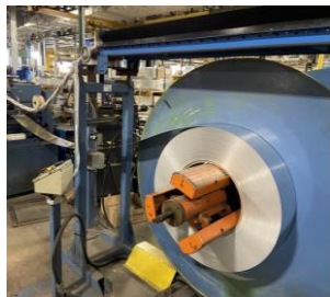
1. Aluminum strip is inserted into the machine in large rolls
