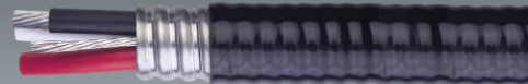
ACW90 Armoured and jacketed cable with 2, 3 or 4 XLPE-insulated Al conductors + bare Al Grd
