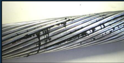
Old Water Blocking Technology – Bitumen
