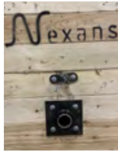
Removable locking device to prevent the reel from rolling.
