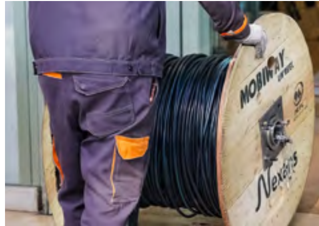
Removable locking device to prevent the reel from rolling.
